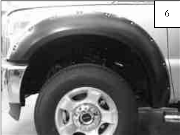
Completed front flare installation.
