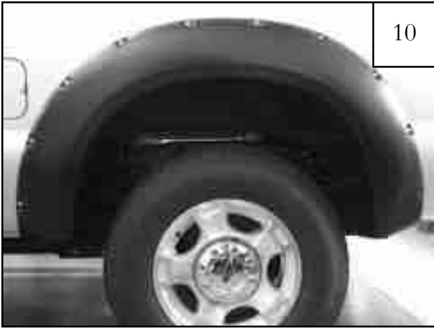
Completed rear flare installation.
