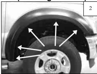
Position flare on fender, lining up factory holes and holes in the flare. Starting with the top, centermost screw, reinstall factory screws through holes in flare and fender with a 7/32" socket wrench.
