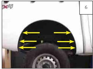
Using a #2 Phillips Screwdriver and or pry tool remove 6 pieces of factory hardware from the rear wheel well and discard. *Note: Some vehicle models will have factory mudflaps. These will need to be removed for proper installation of flares.*
