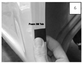
Wrap a Foam Tab (MT1-0034) around the wheel well sheet metal, centered over the mark made in Step 5.
