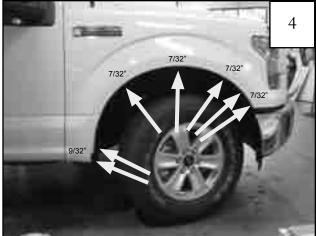
Remove five factory screws with a 7/32" socket wrench. Remove two rear most factory screws with 9/32" socket wrench. Save screws for reinstallation. *Note:* For Platinum Edition, after you remove the factory flare, there are additional screws to be removed. These screws will be used for reinstallation.
