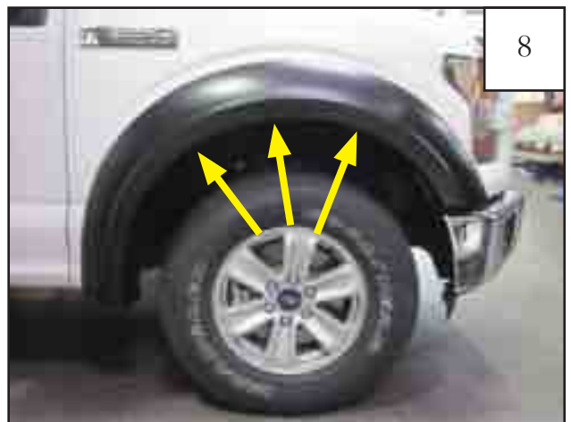
Position flare on fender, pressing inward on the flare, line up the flare mounting holes with the mounting clips on the inner piece. Install 3 Phillips Truss Screws (SW1-0058) through the flare and into the clips on the inner piece. Do not tighten. (3 locations)
