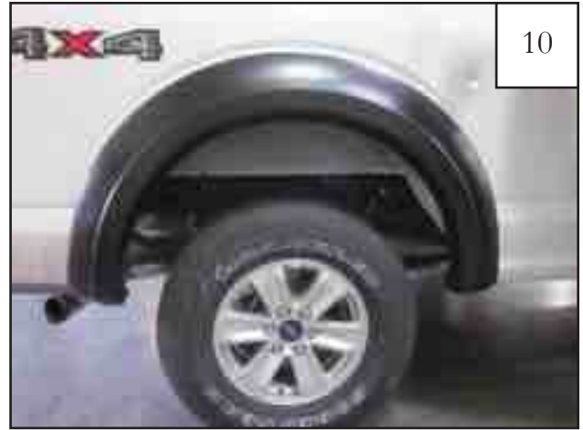
Completed rear flare installation.
