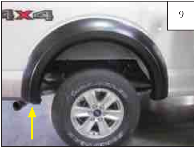
Install supplied push retainer (RV1-P0006) into flare and through factory hole at rear of wheel well.
