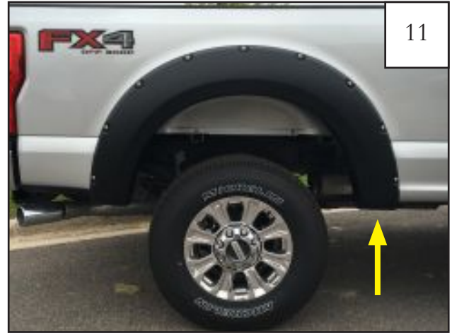
Start a supplied screw (SW1-0050) through the flare into the clip installed in Step 9. Tighten all screws.
