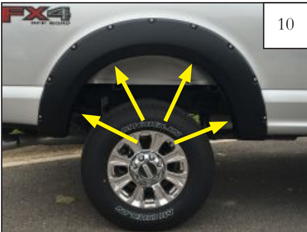
While holding flare to vehicle, start supplied screws (SW1-0058) through the four topmost mounting holes in flare and into the clips installed in Step 8.
