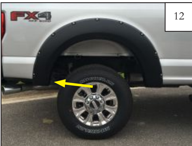
Install supplied push retainer (RV1-P0001) into flare and through factory hole at rear of wheel well.
