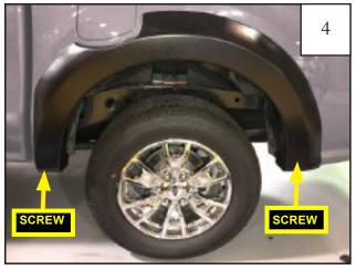
Reinstall (2) T-25 Torx screws previously removed from rear flare in Step 2.
