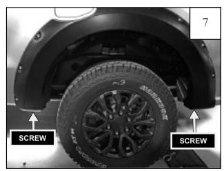
Reinstall (2) T-25 Torx screws previously removed from rear flare in Step 17.
