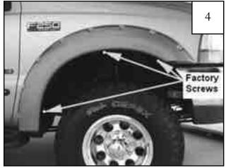
Remove three factory screws with a 7/32" socket wrench. *Save for reinstallation.* Position flare on fender. Apply moderate pressure to outside surface of flare and fasten to vehicle with three factory screws.
