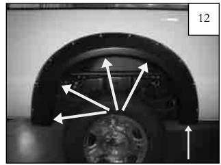
Ensuring proper flare placement, tighten all screws.
