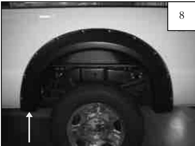
Using a 10mm socket, remove factory hex bolt located at lower front wheel well. Save screws for reinstallation.
