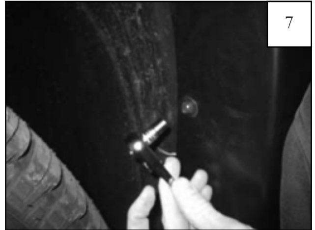
Holding flare in position on fender, reinstall factory screws removed in Step 4.
