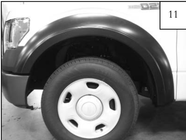
Completed front flare installation.
