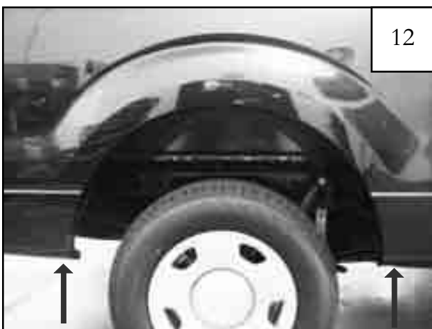
Remove two factory bolts with a 10mm socket wrench. (Note: New hardware is being supplied see Step 17)
