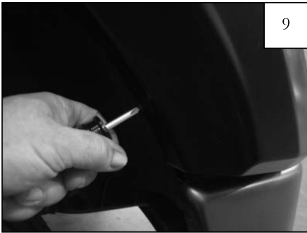
Still holding flare to fender, install supplied black plastic retainers (RV1-P001) using a Phillips screw driver. See step 10.
