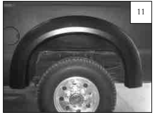
Completed rear flare installation.
