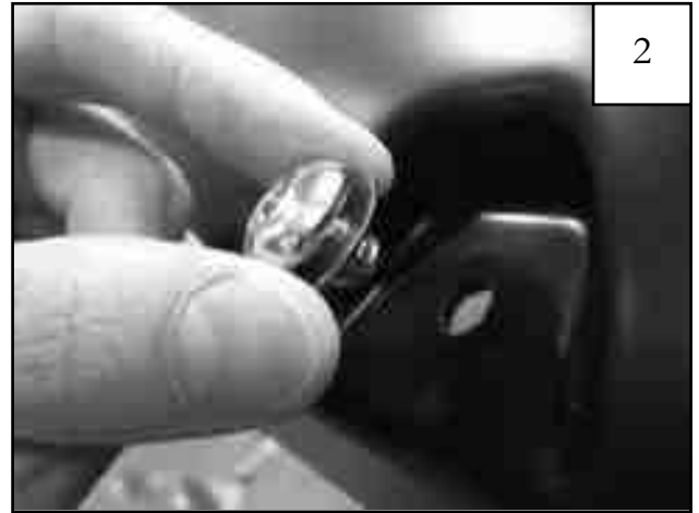
Put each Bolt/Washer combination through a pocket hole in the flare, Bolt head and Washer on the outside.
