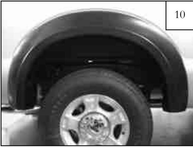
Completed rear flare installation.
