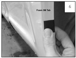
Wrap a Foam Tab (MT1-0034) around the wheel well sheet metal, centered over the mark made in Step 5.
