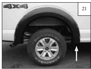
Start a supplied screw (SW1-0050) through the flare into the clip installed in Step19. Tighten all screws.
