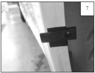
Install a Clip (CL1-0009) over the Tab (MT1-0034) placed in Step 6.
