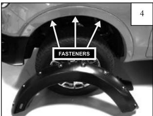
Remove (3) factory installed plastic fasteners from the driver side front wheel well using a phillips screwdriver. Needle nose pliers may be needed to extract the fasteners.
