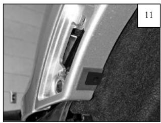
Install (1) "S" spring clip (CL1-0005) over the black mylar tab, centered with the grease pencil marking.
