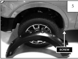
Remove (1) factory installed screw from the rear of the fender trim using a T-25 Torx driver.
