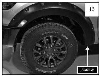
Reinstall (1) T-25 Torx screw previously removed from rear of the flare in Step 5.
