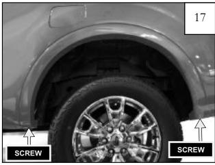
Remove (2) factory installed screws from under the fender trim using a T-25 Torx driver. The screws will be re-used to install the rear flare.
