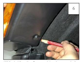
While holding the flare up into place, mark the location of the front hole on the fender liner using a grease pencil.
