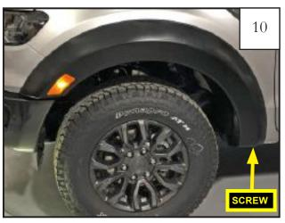
Reinstall (1) T-25 Torx screw previously removed from rear of the flare in Step 2.
