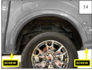
Remove (2) factory installed screws from under the fender trim using a T-25 Torx driver.
