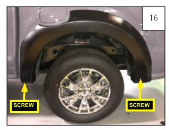
Reinstall (2) T-25 Torx screws previously removed from rear flare in Step 14.
