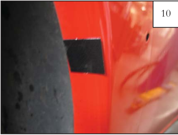
Install a Tab (MT1-0002) centered over mark made in Step 9. Edge of Tab should be even with edge of sheet metal.
