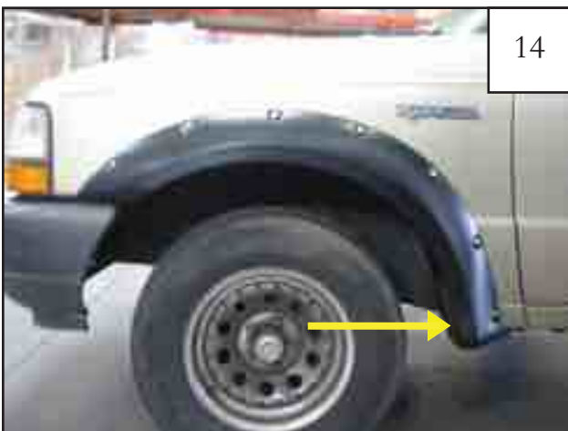
Reinstall factory screw saved from Step 8.
