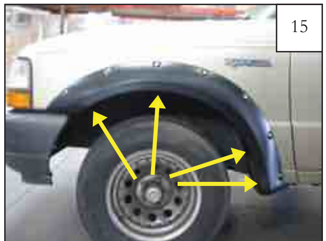
Ensuring proper flare placement, tighten all screws.
