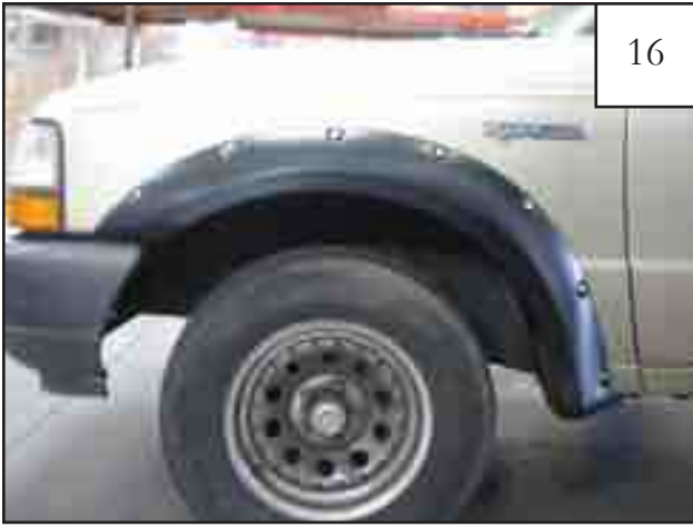
Completed front flare installation.
