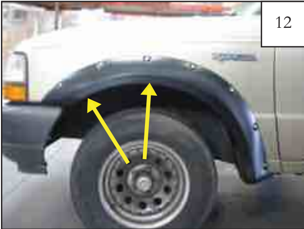
Hold flare in place and start Screws (SW1-0058) in Clip (CL1-0022) locations and into inner piece. Do not tighten.
