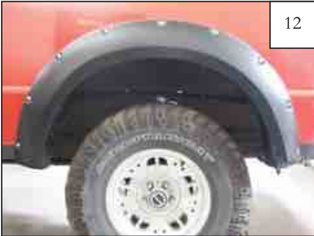
Completed rear flare installation.
