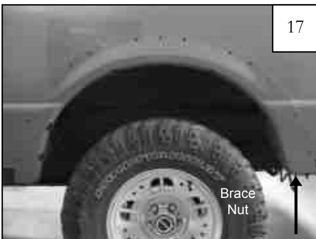
Remove any installed factory flares, mud flaps, or stone guards and clean wheel well opening. Remove rear Fender Brace Nut with a 13mm socket. Save brace nut for reinstallation.
