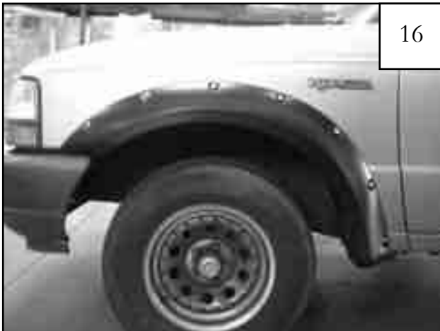
Completed front flare installation.
