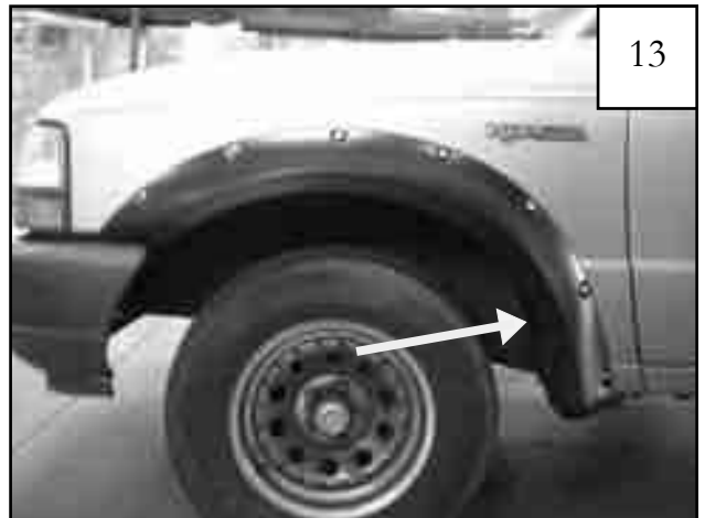
Start Screw (SW1-0050) into Clip (CL1-0006) installed in Step 11. Do not tighten.
