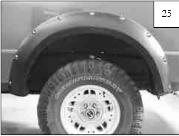
Completed rear flare installation.
