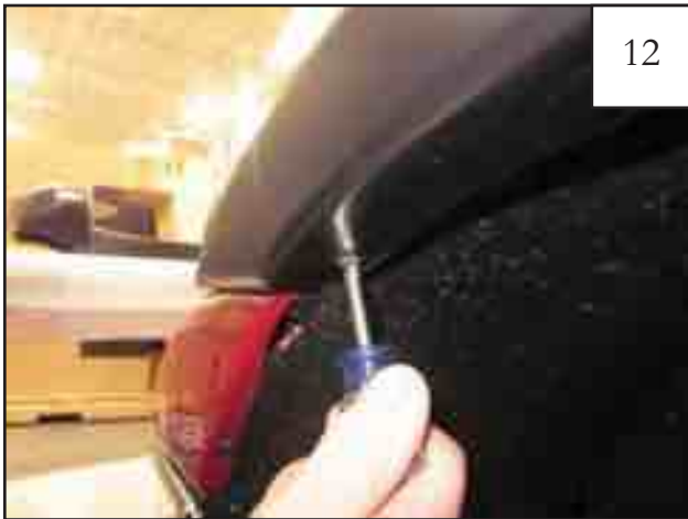
Align holes in flare with holes in Clips (CL1-0005). Start a supplied Screw (SW1-0050) through holes in flare and into each Clip (CL1-0005) installed in Step 11 in the order shown in Step 13. If necessary, use an awl to locate holes in clips.
