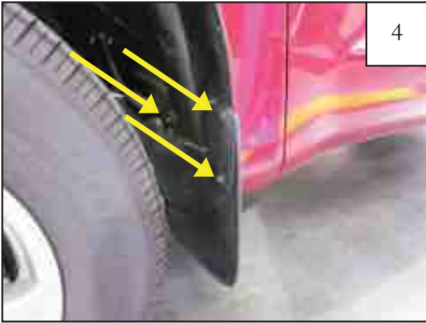
Remove three hex bolts from factory mud flap, using a 10mm socket.
