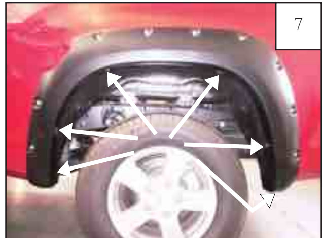
Hold flare firmly on the fender. Start a supplied Screw (SW1-0036) through each hole in flare and into hole in fender. (6 locations)
