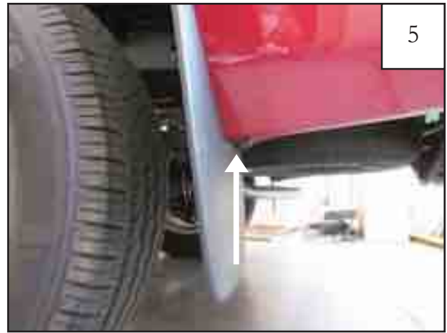
Remove one hex bolt from underside of mud flap using a 10mm socket. Discard mud flap.
