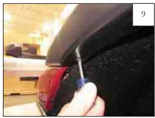
Align holes in flare with holes in Clips (CL1-0005). Start a supplied Screw (SW1-0050) through holes in flare and into each Clip (CL1-0005) installed in Step 11 in the order shown in Step 13. *If necessary, use an awl to locate holes in clips.*
