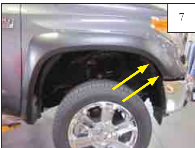
Start two supplied 20mm Hex Screws through front most holes in flare and into factory hole locations.
