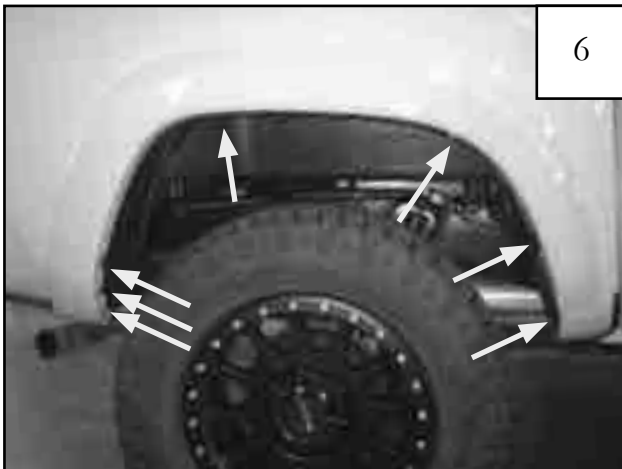
Remove seven factory screws. If there is no factory flare is installed, go to Step 11.
