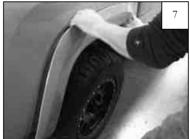
Remove flare by carefully pulling part away from side of vehicle.
