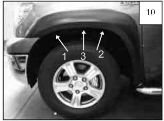
Start Screw (SW1-0050) in location #1 first, then move to #2, and start in location #3 last. **DO NOT TIGHTEN**.
