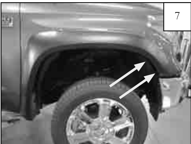
Start two supplied 20mm Hex Screws through front most holes in flare and into factory hole locations.
