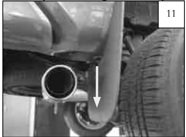
Remove factory push retainer from underside of factory mud guard and remove mud flap.
