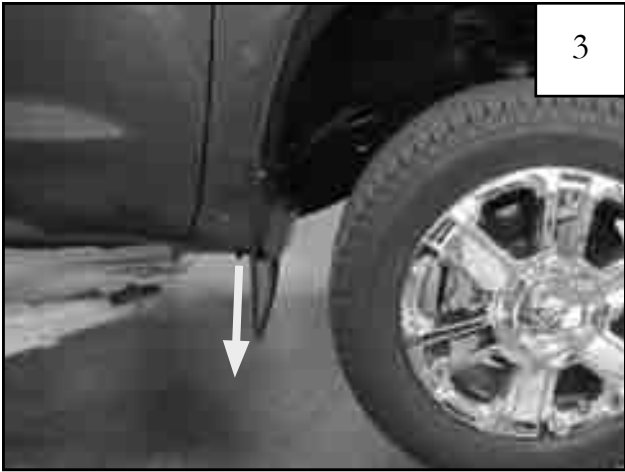
Remove factory push retainer from underside of factory mud guard. Remove Mud Guard from Vehicle.
