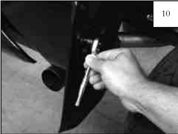
Using a socket wrench with a 10mm socket, remove factory screws from the factory mud guard.
