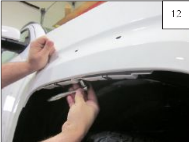
Using three supplied screws (SW1-0036), attach bracket to wheel well. Tighten all screws.
