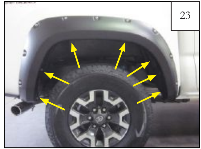
Holding flare to fender, install supplied screws (SW1-0036) into mounting holes (7 places).
