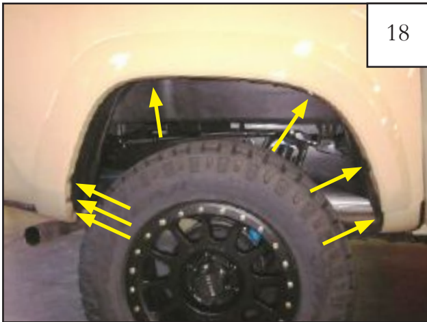
Remove seven factory screws. If there is no factory flare installed, go to Step 23.
