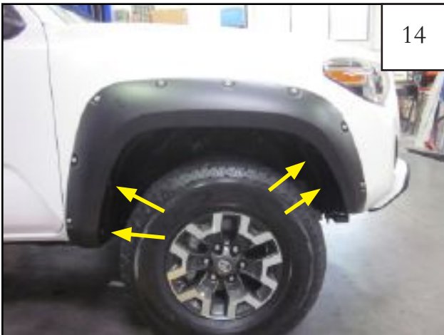
Still holding flare to fender, install supplied screws (SW1-0036) into remaining mounting holes (4 places).
