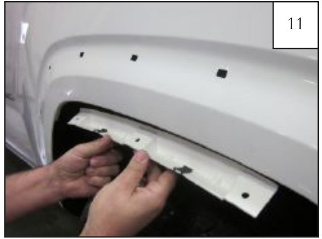
Line up the holes in the inner piece with the three uppermost factory holes. NOTE: Driver's side inner piece is marked with an "LF" and passenger's side inner piece is marked with an "RF"
