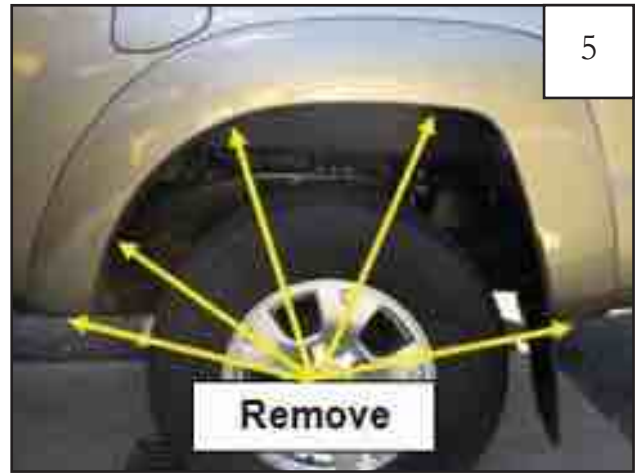
Remove five factory screws. Save screws for reinstallation. Remove flare by pulling part away from side of vehicle.
