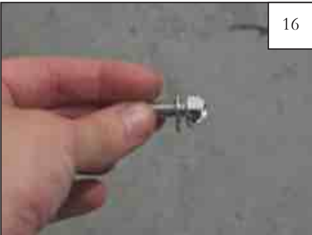
Slide a supplied Washer (WA1-0005) onto a supplied Bolt (SW1-0005).
