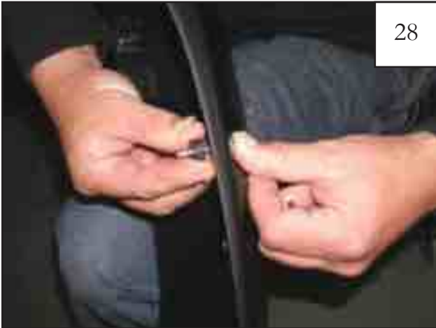
Install Screw/Washer assembly through pocket holes of bumper piece. Place a supplied Spacer (SP1-0011) on the back of the Screw.
