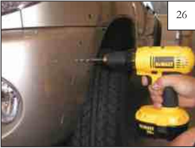
Remove fasteners installed in steps 23 - 24 and remove flare from fender. Drill at marked places with a 5/16" drill bit.
