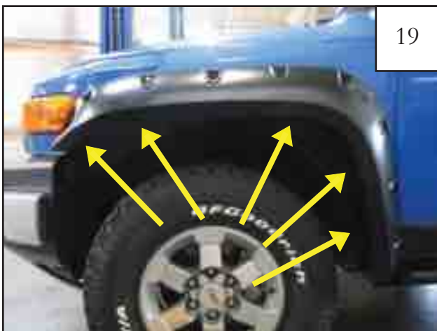
Position Flare on fender. Install five supplied Screws (SW1-0036). Do not tighten. NOTE: It is helpful to install one of the top bolts first.
