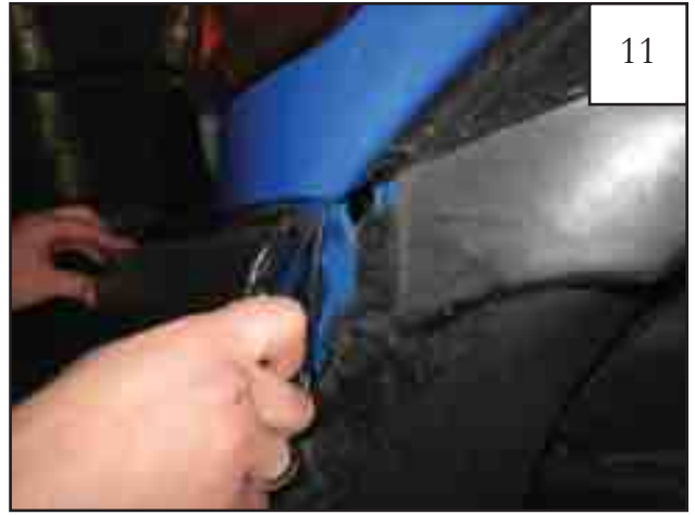
Trim remaining plastic flush with bumper.
