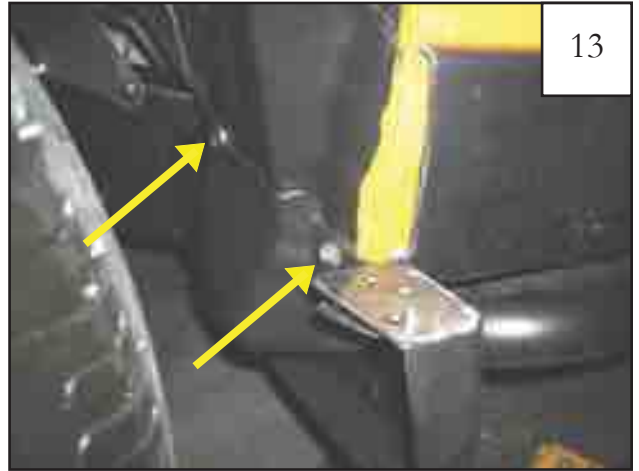
Remove mud flap bolts as shown (2 places).
