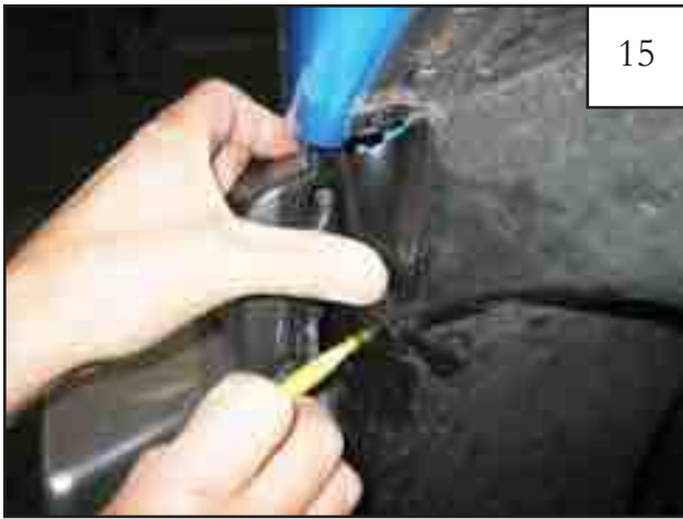
Holding Front Inner Piece on front of wheel well next to bumper, use a grease pencil to mark two clip locations.
