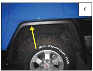
Using a pry tool or flat head screwdriver, remove one plastic fastener.
