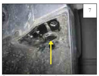
Remove one plastic fastener from mud guard.
