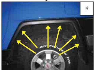
Using a 10mm socket, remove six bolts.
