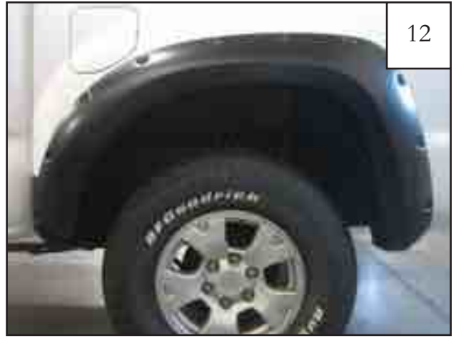
Completed rear flare installation.
