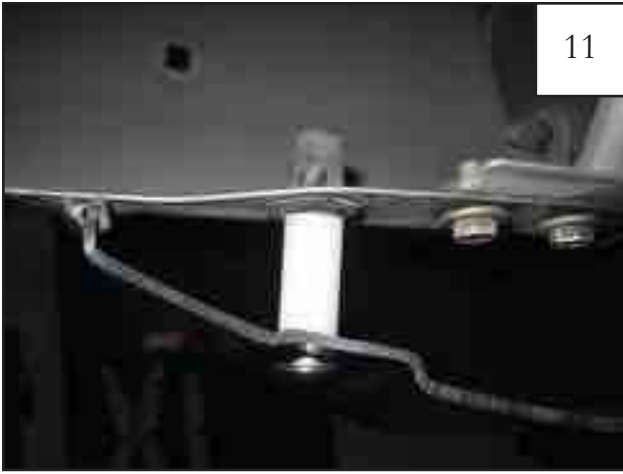
At bottom rear of flare, fasten flare to vehicle with a supplied 1-3/4" #14 Truss Head Screw (SW1-0034) through a 1" Spacer (SP1-0005).
