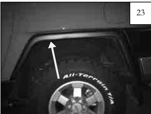
Using a pry tool or flat head screwdriver, remove one plastic fastener.
