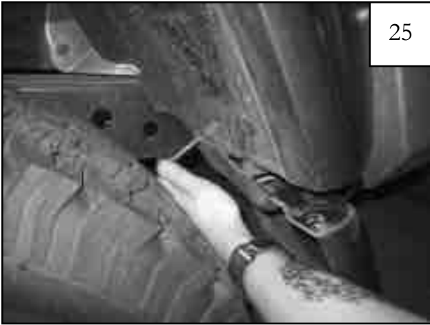
Remove bolt from mud guard located inside wheel well.
