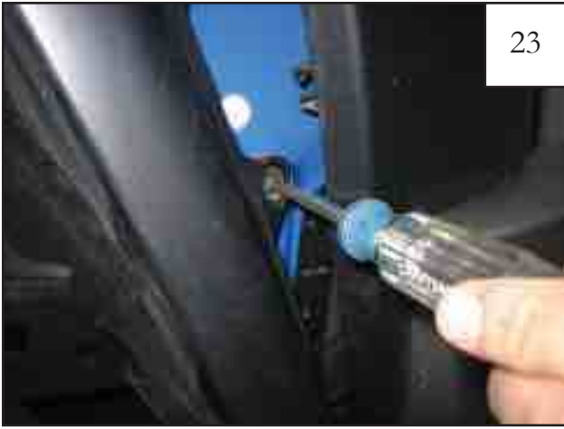
Remove bolt located behind rear plastic panel. Note: If the socket does not fit in the enclosed space, a phillips screwdriver will work.
