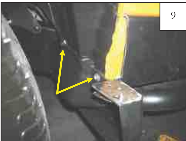
Remove mud flap bolts as shown in image above (2 places).
