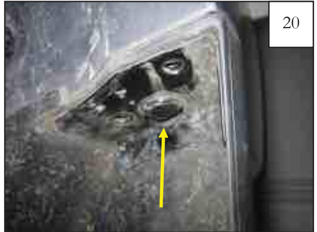
Remove one plastic fastener from mud guard.
