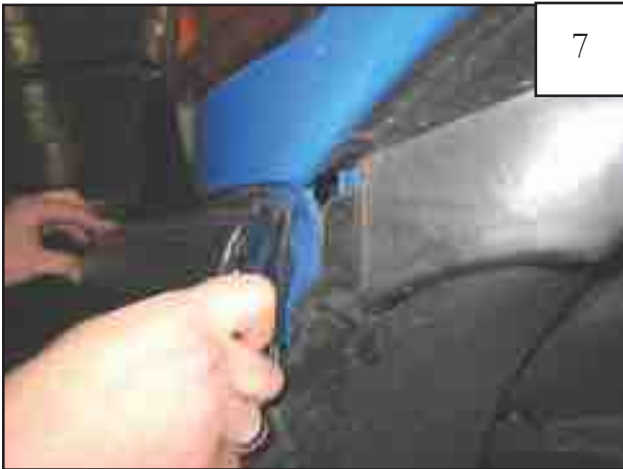
Trim remaining plastic flush with bumper.
