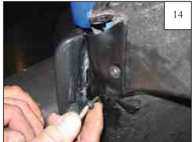
Position Inner Front Piece on vehicle, aligning holes in part with holes in clips installed in Step 13. Install supplied Pan Head Screws
