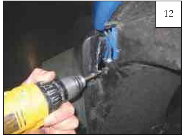
Remove Front Inner Piece and drill two 5/16" holes on marks made in Step 11.
