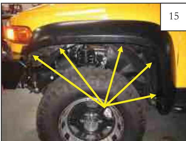
Position Flare on fender. Install five supplied #14 Hex Head Bolts. Do not tighten at this time. Note: It is helpful to install one of the top bolts first.
