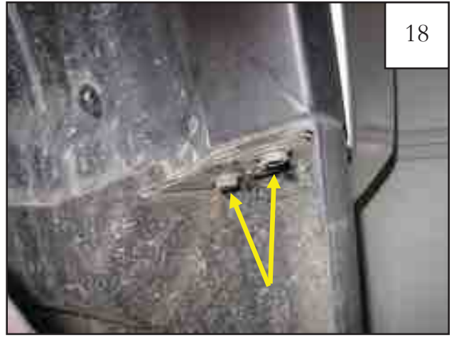
Remove two factory bolts from mud flap.
