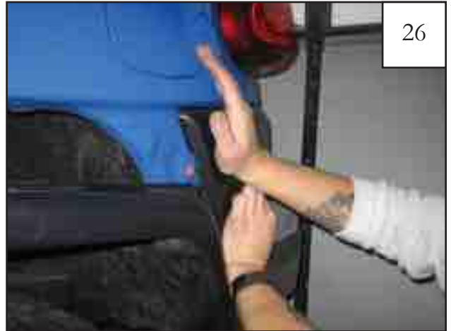
Remove bolt from underside of factory flare (behind panel). Pry flare from fender, releasing plastic clips.
