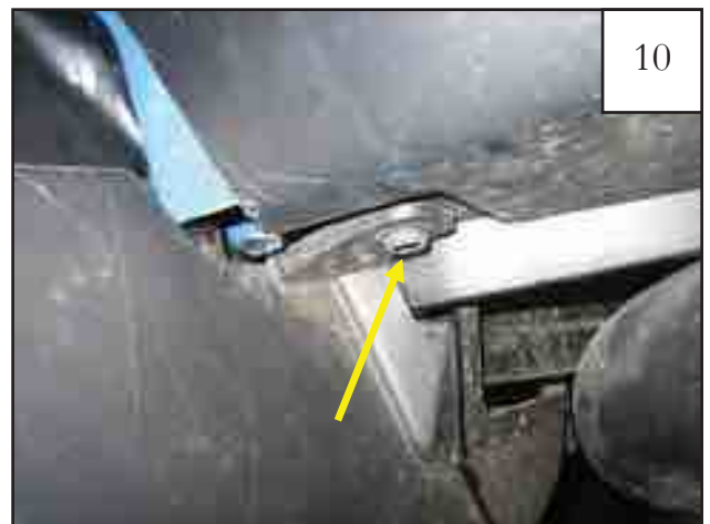
Remove the third mud flap bolt, and remove mud flap.
