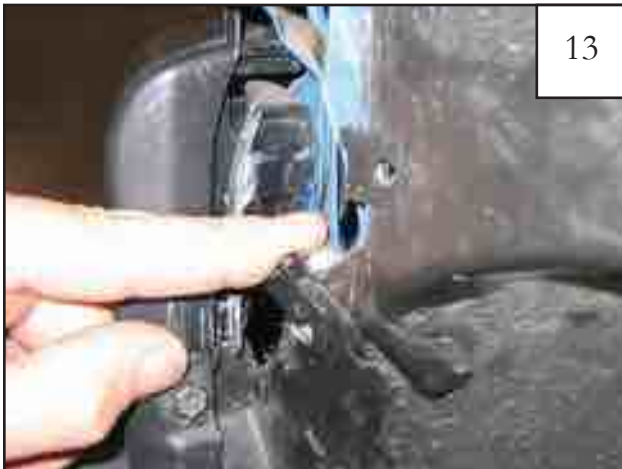
Slide the supplied "U" Clips over holes drilled in Step 12 (2 places). Note: Some trimming of plastic may be required for correct clip alignment.
