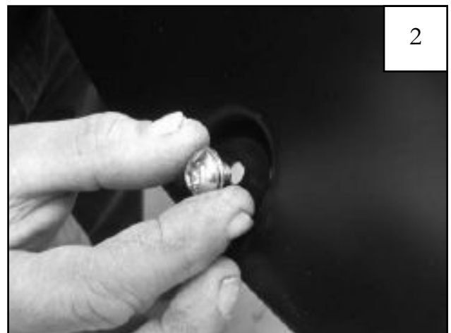
FRONT MAIN & REAR FLARE ONLY: Put each Bolt/Washer combination through a pocket hole in the flare, Bolt head and Washer on the outside. See Steps 36 - 38 for installation with an Aftermarket Bumper.
