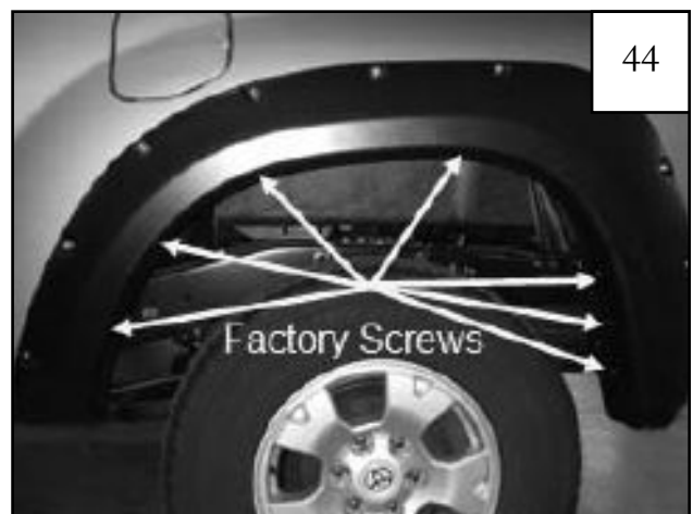
Position flare on fender and install seven factory fasteners through holes in flare and into factory holes.
