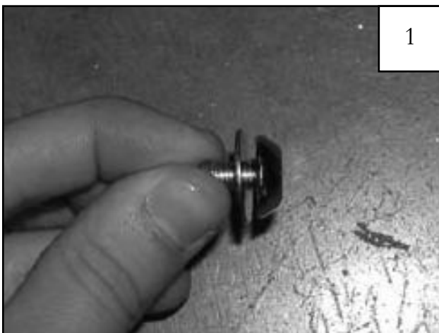
Put a Washer (WA1-0007) on each Bolt (SW1-0032).
