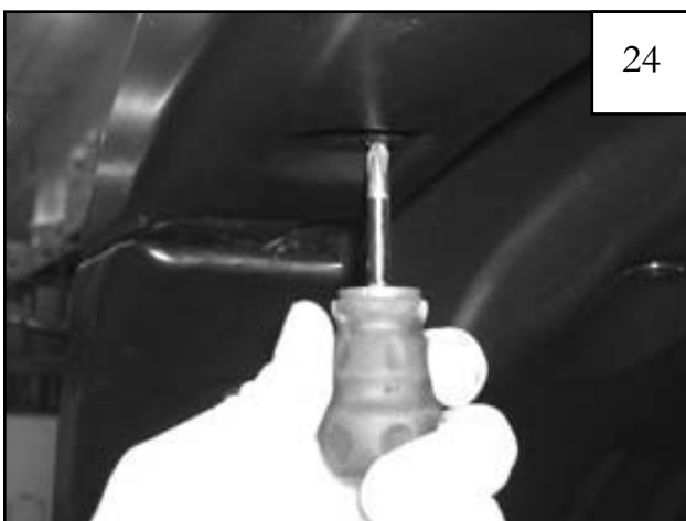
Install a supplied Screw (SW1-0050) through hole in flare and into Clip installed in step 22. 4 places.
