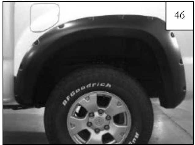
Completed rear flare installation.
