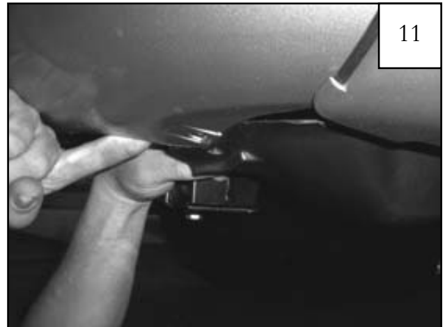
Pull down bumper cover and splash shield.
