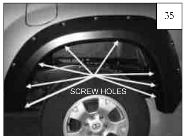
Position flare on fender and install eight supplied hex head screws (SW1-0036) through holes in flare and into factory holes.
