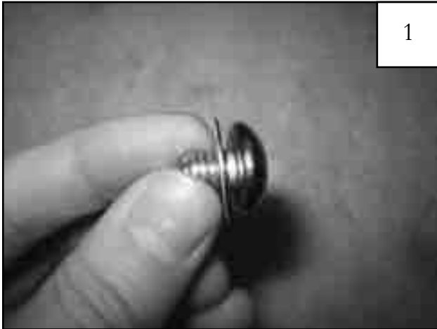
Put a Washer (WA1-0010) on each Bolt (SW1-0059).
