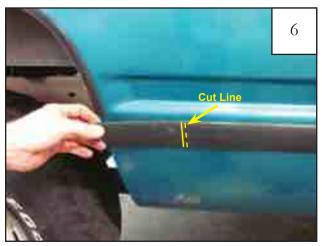
Remove the flare and mark a cut line 1/4" beyond overlap line. Use blow dryer or heat gun to heat molding.
