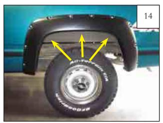
Ensuring flare is proplery located on fender, start supplied screws (SW1-0050) through each of the remaining holes.
