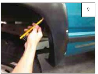
Hold flare in position on fender using moderate pressure. Using a grease pencil, mark five hole locations using the holes in the flare as a guide. (See Step 10)
