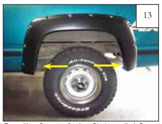
Reposition flare on fender. Start supplied Screw (SW1-0050) through two corner hole locations and through each Clip (CL1-0005) installed in step 12. If needed, use awl to align holes with the installed clips.
