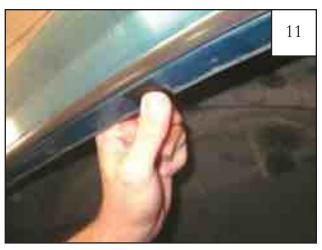
Remove flare. Center a supplied Tab (MT1-0002) over the marks made in step 10, aligning edge of tab with inside edge of fender lip (tab may extend over outside of fender).
