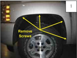
Using a 7mm socket, remove factory screws. Set aside for reinstallation.
