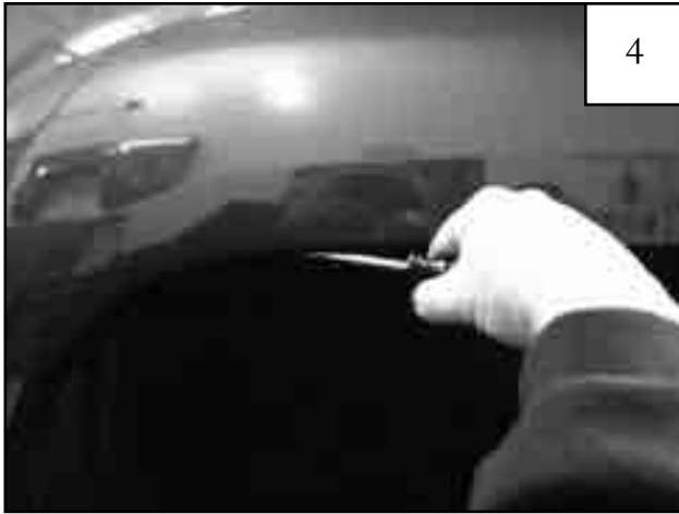
For 2011-UP ONLY: Using a pry tool remove factory installed tufflocs .
