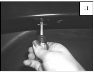
Reposition flare on fender, Start a supplied Screw (SW1-0057) through the two uppermost holes in the flare and into each Clip installed in Step 6.
