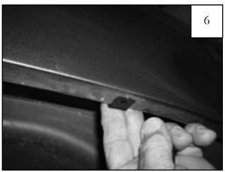
Center a supplied Clip (NU1-0007) over the upper two marks made in Step 4. Clips may need to be adjusted to align with holes in flare. *Note: The raised* collar on the Clip should face upward into the interior of the fender.
