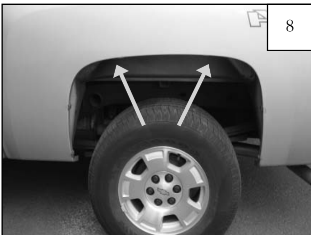
Slide a supplied Clip (CL1-0022) over tabs installed in step 7. Clips may need to be adjusted to align with holes in flare. Note: Some vehicles with inner splash shield will need to remove factory fasteners in indicated locations before installing the clips.
