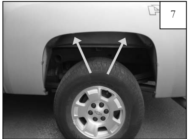
Center a supplied Tap (MT1-0002) over top two factory holes.
