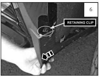
Firmly pull the mud flap away from vehicle in order to disengage the factory retaining clip, and remove mudflap from vehicle. If necessary, pliers may be needed to squeeze clip from behind.
