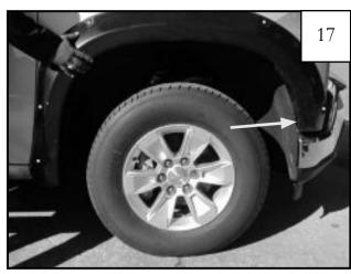
Install (1) supplied phillips head screw (SW1-0049) at front Clip location. *Do not tighten*. (If needed use an awl to align flare mounting holes.)
