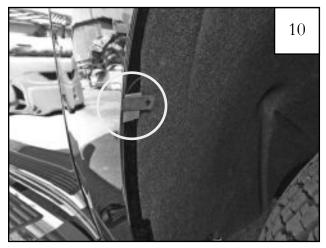
Install supplied Tab (MT1-0034) over the rear location marked in Step 9. Install a Clip (CL1-0009) as indicated on top of the protective film.
