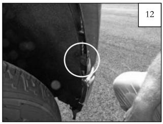
Install supplied Tab (MT1-0017) over the front location marked in Step 9. Install a clip assembly as indicated, on top of the Tab. See Step 13 for detail of clip attachment.
