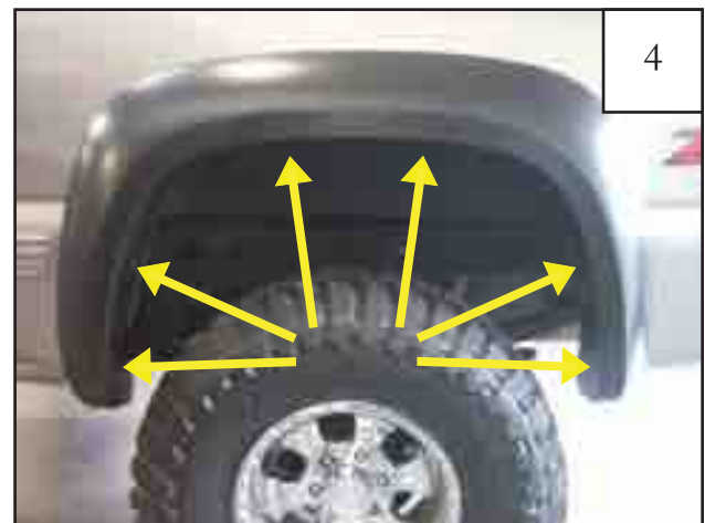
Install six tuflocks using a #2 stubby screwdriver.
