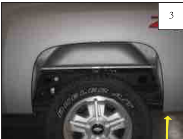
Remove one factory bolt with a 1/2" wrench.
