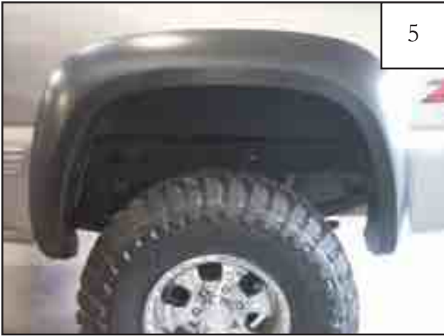
Completed rear flare installation.
