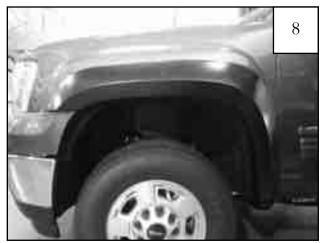
Completed front flare installation without bumper piece.
