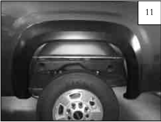
Completed rear flare installation.
